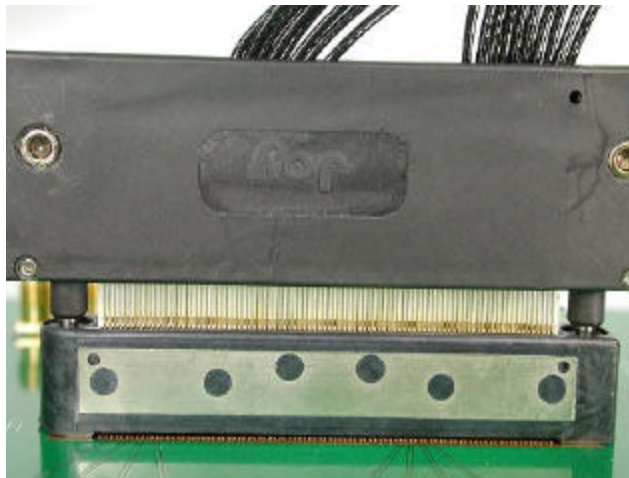
Figure 2a) Close-up of male-to-female connection
