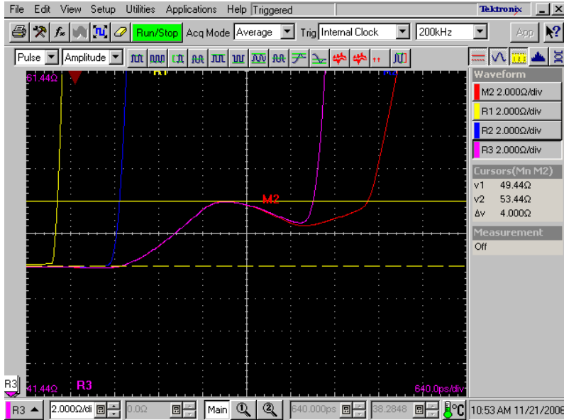
Figure 5) Same trace as Figure 1 except with a 1ns risetime (20-80%) filter applied. The vertical scale has been enlarged showing an impedance variation of 4 ohms.
