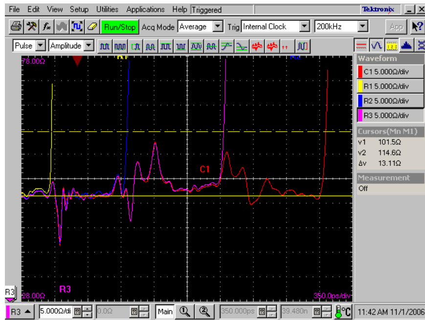
Figure 9) Impedance of 6 inch double-ended cable assembly and top trace on the microstrip test boards taken from end of test lead to end of SMA on second board. First open (yellow) is the end of test lead. Second open (blue) is the end of female ZIF connector on the first board. Third open (purple) is the end of the cable assembly disconnected from the second test board, and fourth open (red) is the end of the second board (at the SMA)
